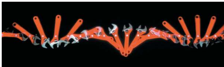
FIGURE 8.23 The center of mass of the spinning wrench follows a straight-line path.
