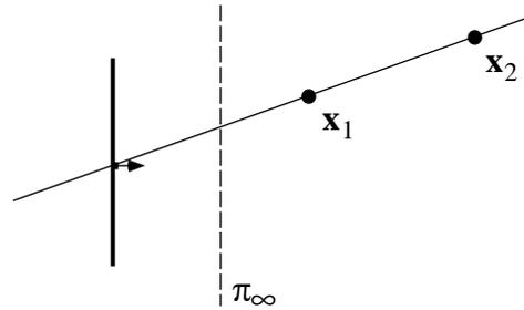
Fig. 21.4. As shown, the point  $\mathbf{x}_1$  is closer to the camera than  $\mathbf{x}_2$ . However, if an orientation-reversing projectivity is applied, taking  $\pi_\infty$  to infinity, then both  $\mathbf{x}_1$  and  $\mathbf{x}_2$  remain in front of the camera, but  $\mathbf{x}_2$  is closer to the camera than  $\mathbf{x}_1$ .
