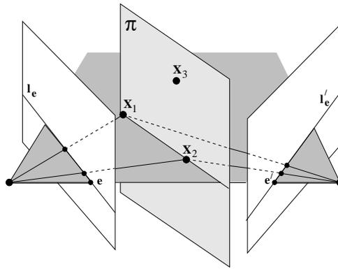
Fig. 13.3. **Degenerate geometry for an implicit computation of the homography.** The line defined by the points  $X_1$  and  $X_2$  lies in an epipolar plane, and thus intersects the baseline. The images of  $X_1$  and  $X_2$  are collinear with the epipole, and  $H$  cannot be computed uniquely from the correspondences  $x_i \leftrightarrow x'_i, i \in \{1, \dots, 3\}, e \leftrightarrow e'$ . This configuration is not degenerate for the explicit method.
