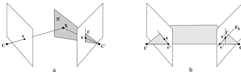
Fig. 13.6. **A degenerate homography.** (a) The map induced by a plane through the second camera centre is a degenerate homography  $H = [l']_x F$ . The plane  $\pi'$  intersects the second image plane in the line  $l'$ . All points in the first view are mapped to points on  $l'$  in the second. (b) A point  $x$  in the first view is imaged at  $x'$ , the intersection of  $l'$  with the epipolar line  $Fx$  of  $x$ , so that  $x' = l' \times Fx$ .
