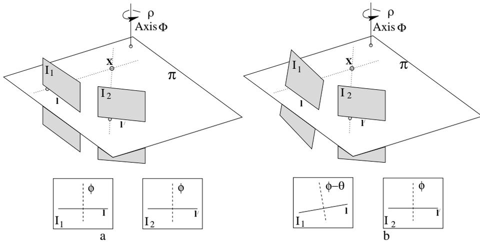
Fig. 14.11. The camera rotates about the axis  $\Phi$  which is parallel to the image plane. The intersection of the epipolar plane  $\pi$  with the image planes gives epipolar lines  $l$  and  $l'$ , and the projections of  $\Phi$  in the images are orthogonal to these epipolar lines: (a) no cyclotorsion occurs ( $\theta = 0^\circ$ ); (b) the camera counter-rotates by  $\theta$  in  $I_1$ , so the orientation of the epipolar lines changes by  $\theta$ .
