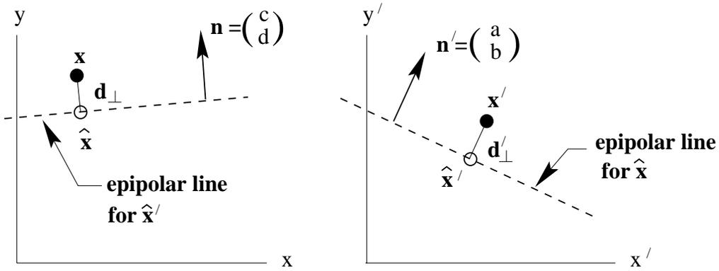
Fig. 14.3. The MLE of  $F_A$  from a set of measured corresponding points  $\{\mathbf{x}_i \leftrightarrow \mathbf{x}'_i\}$  involves estimating the five parameters  $a, b, c, d, e$  together with a set of correspondences  $\{\hat{\mathbf{x}}_i \leftrightarrow \hat{\mathbf{x}}'_i\}$  which exactly satisfy  $\hat{\mathbf{x}}'_i{}^T F_A \hat{\mathbf{x}}_i = 0$ . There is a linear solution to this problem.
