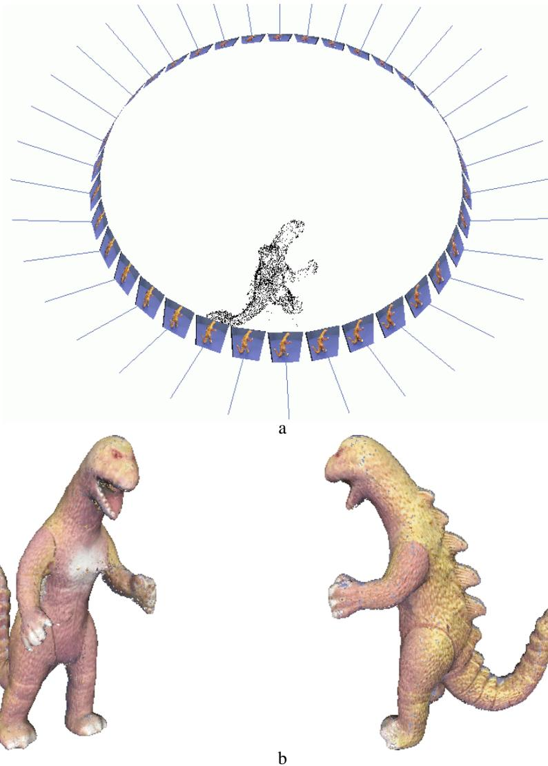
Fig. 19.8. **Dinosaur:** (a) 3D scene points (about 5000) and camera positions for the Dinosaur sequence. (b) The automatic computation of a 3D graphical model for this sequence is described in [Fitzgibbon-98b].
