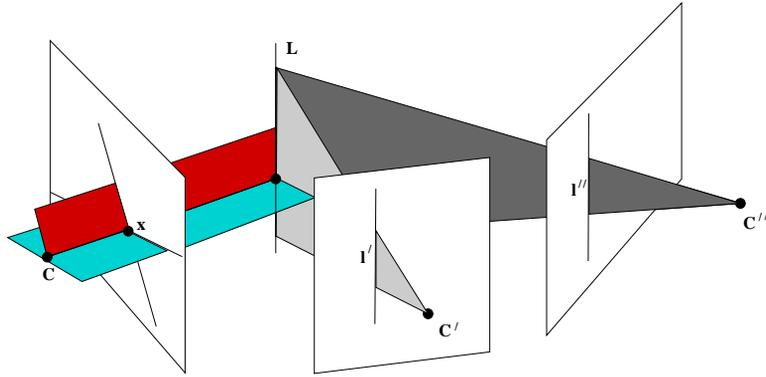
Fig. 17.2. A point–line–line correspondence  $\mathbf{x} \leftrightarrow \mathbf{l}' \leftrightarrow \mathbf{l}''$  involving three images may be interpreted as follows. Two arbitrary lines are chosen to pass through the point  $\mathbf{x}$  in the first image. The four lines then back-project to planes that meet in a point in space.
