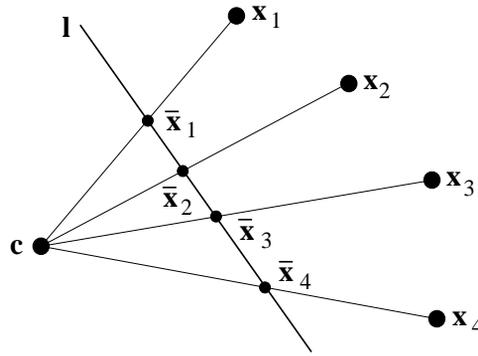
Fig. 22.1. Projection of points in the plane using a 2D camera. A 1D image is formed by the intersection of the rays  $\mathbf{l}_i = \overline{c\mathbf{x}_i}$  with the image line  $\mathbf{l}$ . The set of image points  $\{\bar{\mathbf{x}}_i\}$  is projectively equivalent to the set of rays  $\{\mathbf{l}_i\}$ . For four points, the projective equivalence class of the image is determined by the cross ratio of the points.
