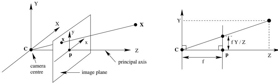
Fig. 6.1. **Pinhole camera geometry.**  $\mathbf{C}$  is the camera centre and  $\mathbf{p}$  the principal point. The camera centre is here placed at the coordinate origin. Note the image plane is placed in front of the camera centre.
