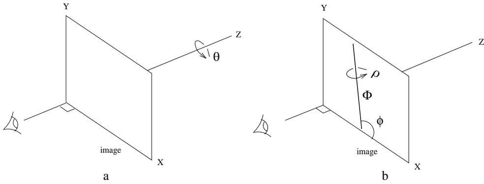
Fig. 14.10. **The rotation representation.** (a) rotation by  $\theta$  about the Z-axis; (b) subsequent rotation by  $\rho$  about a fronto-parallel axis  $\Phi$  angled at  $\phi$  to the X-axis. The  $\Phi$ -axis has components  $(\cos \phi, \sin \phi, 0)^T$ .
