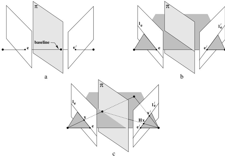
Fig. 13.2. **Compatibility constraints.** The homography induced by a plane is coupled to the epipolar geometry and satisfies constraints. (a) The epipole is mapped by the homography, as  $e' = He$ , since the epipoles are images of the point on the plane where the baseline intersects  $\pi$ . (b) Epipolar lines are mapped by the homography as  $H^T l'_e = l_e$ . (c) Any point  $x$  mapped by the homography lies on its corresponding epipolar line  $l'_e$ , so  $l'_e = Fx = x' \times (Hx)$ .
