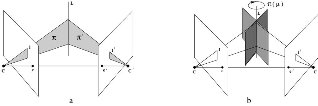
Fig. 13.4. (a) Image lines  $l$  and  $l'$  determine planes  $\pi$  and  $\pi'$  respectively. The intersection of these planes defines the line  $L$  in 3-space. (b) The line  $L$  in 3-space is contained in a one parameter family of planes  $\pi(\mu)$ . This family of planes induces a one parameter family of homographies between the images.
