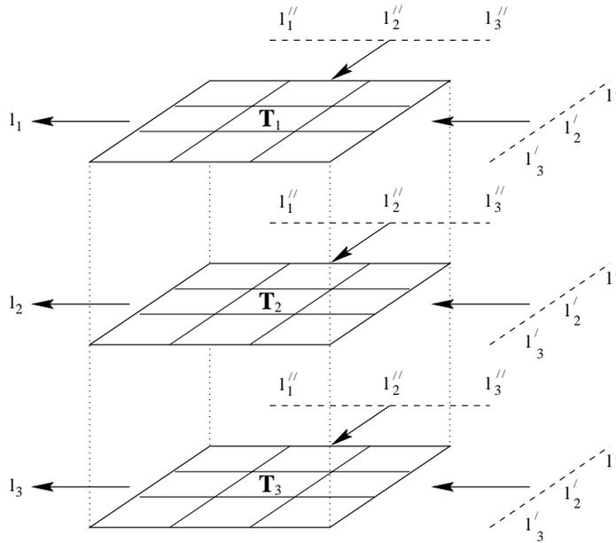
Fig. A1.1. **A 3-dimensional representation of the trifocal tensor** – figure after Faugeras and Papadopoulos [Faugeras-97]. The picture represents  $l_i = l'_j l''_k T_i^{jk}$ , which is the contraction of the tensor with the lines  $l'$  and  $l''$  to produce a line  $l$ . In pseudo-matrix notation this can be written as  $l_i = l'^T T_i l''^T$ , where  $(T_i)_{jk} = T_i^{jk}$ .
