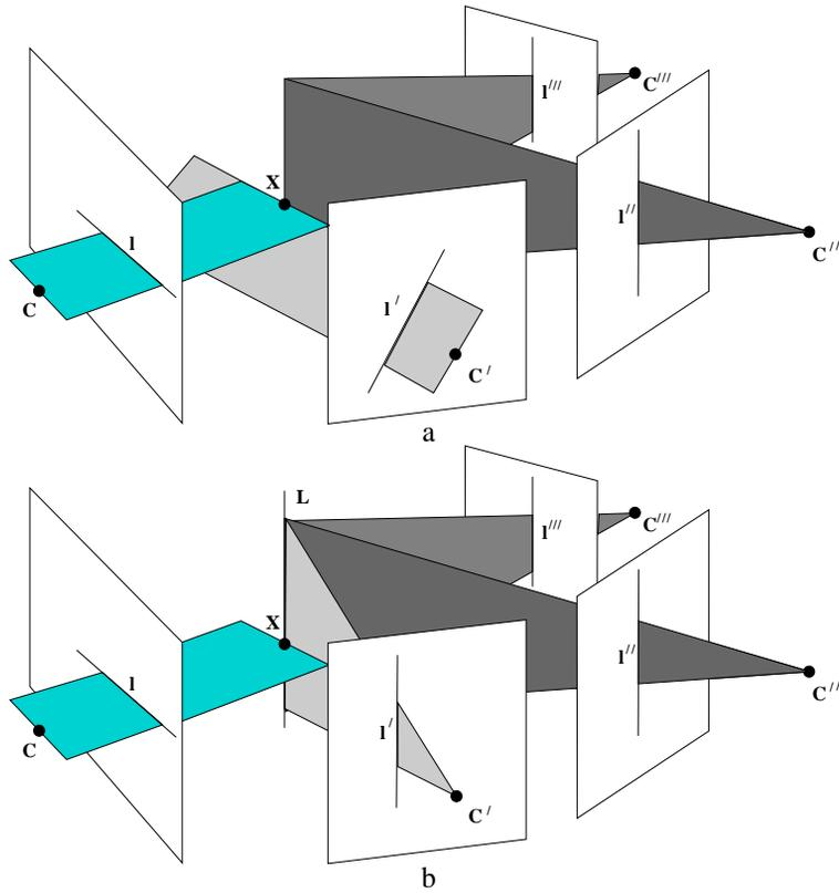
Fig. 17.1. **Four line “correspondence”**. The four lines  $l, l', l'', l'''$  satisfy the quadrilinear relation (17.22) since their back-projections intersect in a common point  $X$ . (a) No three planes intersect in a common line. (b) The three lines  $l' \leftrightarrow l'' \leftrightarrow l'''$  are the image of the same line  $L$  in 3-space.
