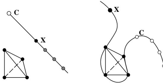
Fig. 22.5. **Left:** Any point on the line passing through  $C$  and  $X$  is projected to the same point from projection centre  $C$ . **Right:** The dual statement – from any centre of projection  $C$  lying on a twisted cubic passing through  $X$  and the vertices of the reference tetrahedron, the five points are projected in the same way (up to projective equivalence). Thus a camera is constrained to lie on a twisted cubic by its image of five known points.
