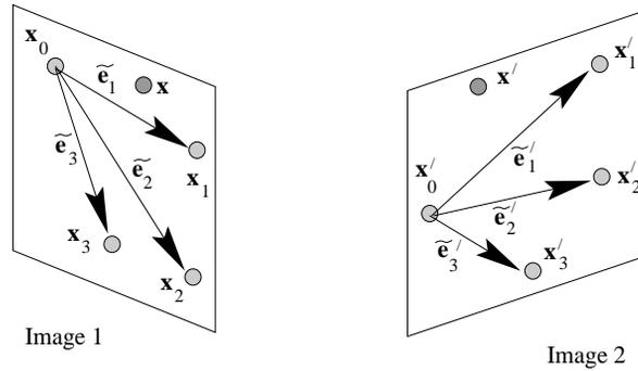
Fig. 14.7. **Reconstruction from two images.** The affine coordinates of the 3D point  $X$  with image  $x, x'$  in two views may be computed linearly from the projection of the basis points  $x_i$  and basis vectors  $\tilde{e}_i$  of figure 14.6.
