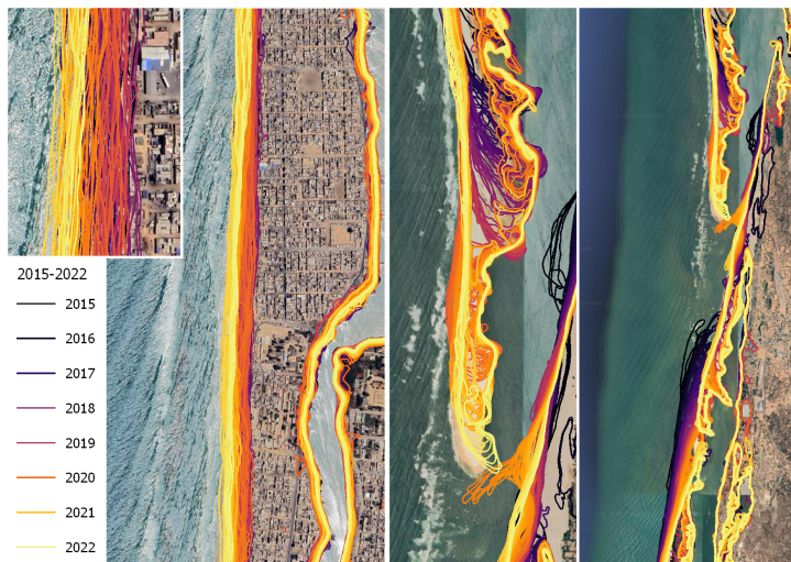
Saint Louis area shoreline detection over time, from Landsat and Sentinel-2 missions. (from Bergsma et al., 2023)
