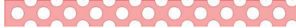
Figure 3 Homogeneous medium whose dimensions are L=0.05625\text{m} , l=0.005\text{m} the cylinders have a diameter of 0.0025\text{m} .
