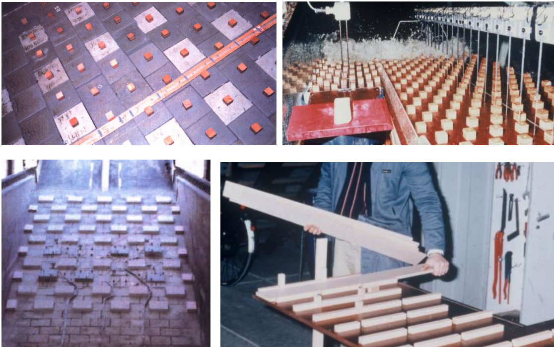
Figure 5.25: Artificial roughness by blocks and battens or ribs. Fig. a: blocks covering 1/25 of surface; Fig. b: blocks covering 1/9 of surface; Fig. c: blocks 8 cm higher for ¼ of surface; Fig. d: preparing battens or ribs on smooth surface for testing
