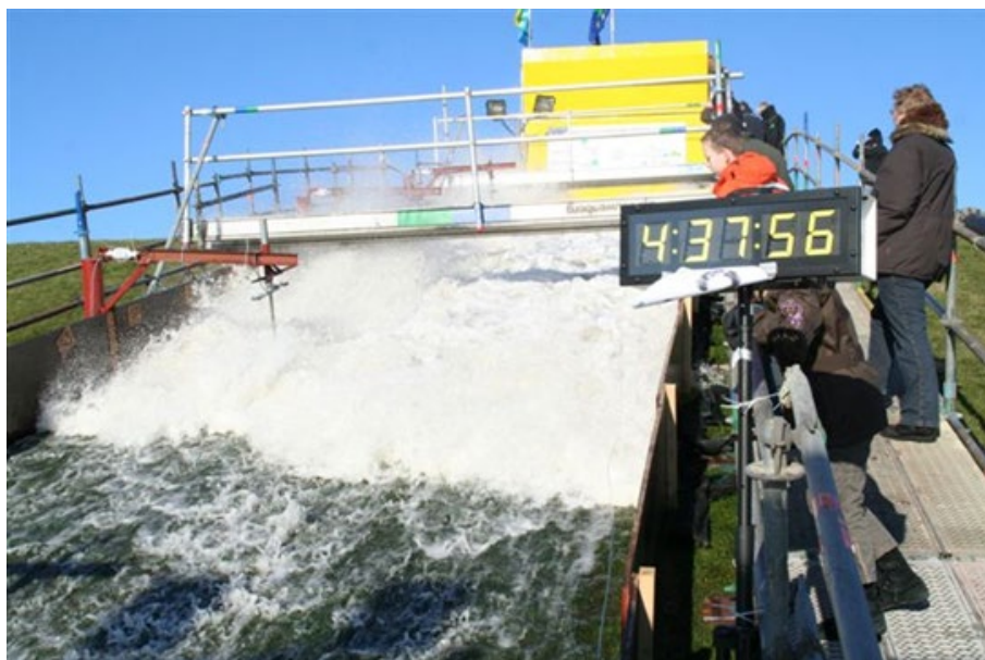
Figure 4.34 Release of a large overtopping wave volume
