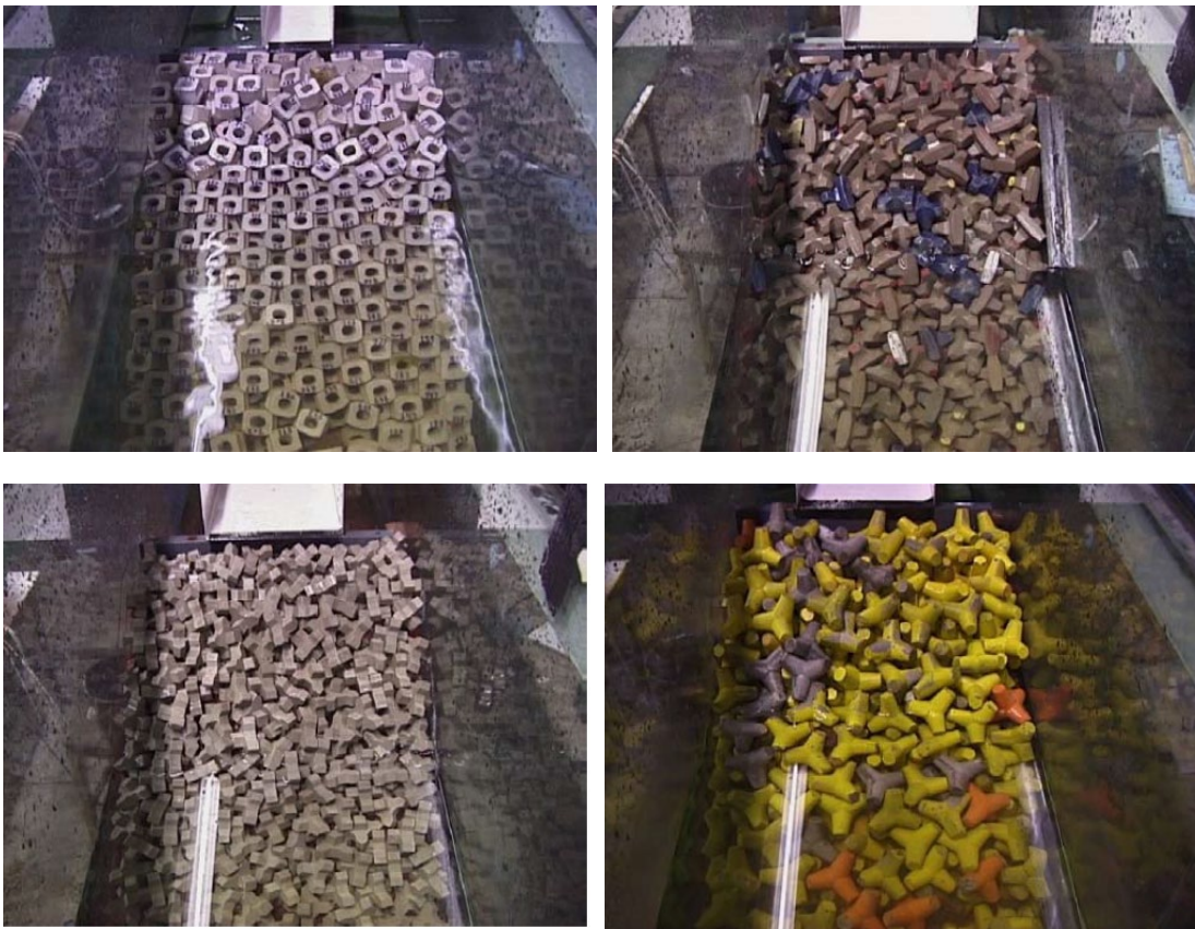
Figure 6.9: Clockwise from top left: Haros, Accropode I, Xbloc and Tetrapods; Test set-up in CLASH
