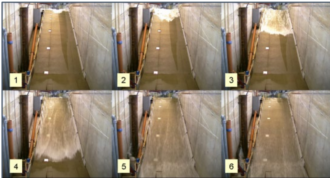
Figure 5.68: Overtopping flow on the landward slope (Large Wave Flume, Hannover)
