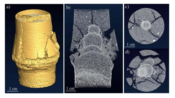
Fig. 5. X-ray tomography images of sample ADA-1; a) 3D view of the fractured sample; b) 2D frontal cross-section, and c) and d) 2D transverse cross-sections showing five different evaporation fronts where halite precipitation has occurred (light grey levels) and the radial fracture network (dark grey levels). Images c) and d) are obtained at around 1.3 and 3 cm from the top of the sample, respectively.
