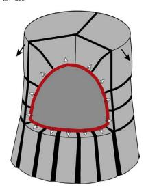
**Fig. 10.** Interpretative sketch of the parabolic evaporation interface that produce local overpressure (white arrows) and fracturing processes that induce secondary sets of radial fracture networks (black) perpendicular to the fracturing-sealing front. Black arrows indicate displacement of fractured blocks.
