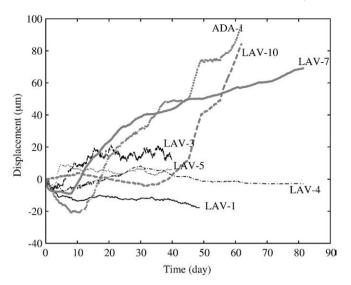
**Fig. 4.** Height of the sample as a function of time during salt capillary rise and precipitation. Samples that have intensively fractured (thick grey lines) show a vertical dilation up to  $100 \, \mu m$ , whereas for samples that did not fracture (fine black lines), no significant deformation could be measured.
