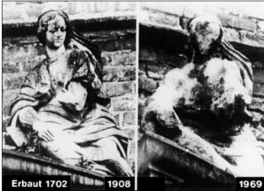
Figure 1. Example of erosion accelerated by atmospheric pollution. Statue carved in 1702 that was in excellent condition in a photo taken in 1908, but had lost all facial features by 1969. Reproduced by permission from Reference 3.
